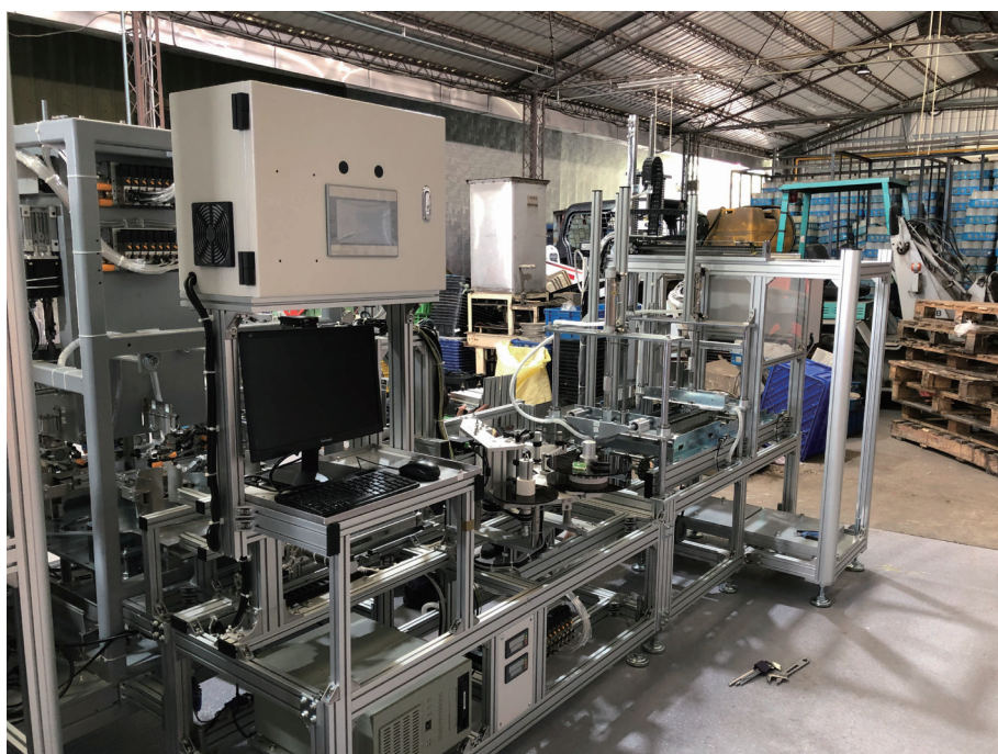
▲ Innovative PP bag-packaging equipment with the production history traceable module
